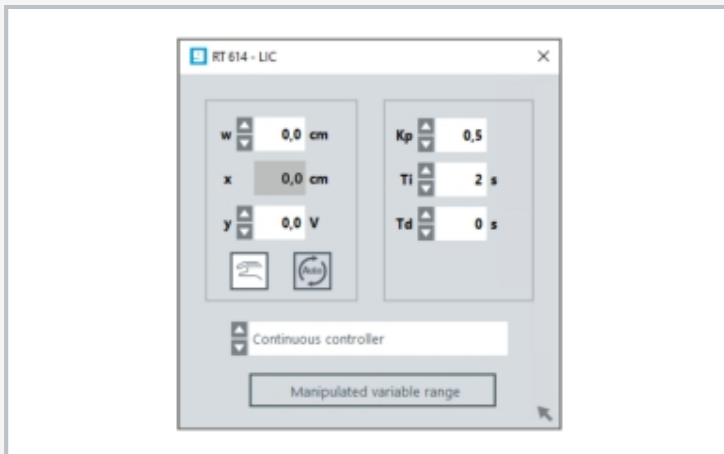
Screenshot: level control demonstration unit RT 614
