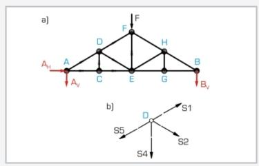
Free-body diagram of a truss:
