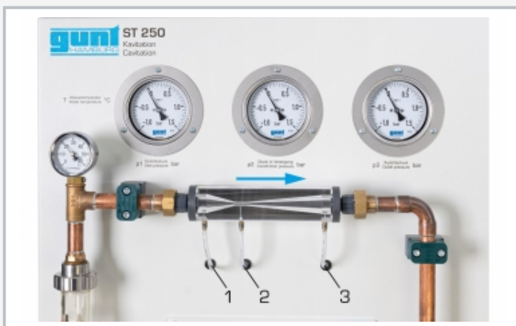
Pressure measurement at the Venturi nozzle with 3 measuring points and manometers: p_1 pressure at the inlet, p_2 pressure at the narrowest cross-section, p_3 pressure at the outlet; blue arrow: flow direction
