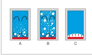
Different modes of boiling: A free convection boiling, B nucleate boiling, C film boiling; red: heater, blue: evaporating liquid, white: steam, black: convection flow
