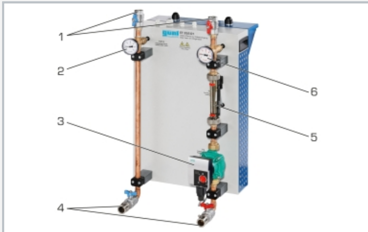
1 feed/return line ET 352, 2 return line thermometer, 3 circulating pump, 4 feed/return line HL 313, 5 flow rate sensor, 6 feed line thermometer
