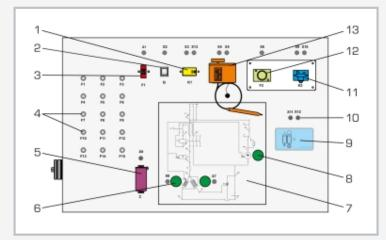
1 main contactor, 2 main switch, 3 automatic fuse, 4 buttons for faults, 5 start-up capacitor, 6 lamp for simulated compressor, 7 circuit diagram, 8 lamp for simulated fan, 9 fan switch, 10 lab jacks, 11 start-up relay, 12 overheat protection, 13 thermostat
