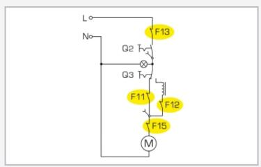
Faults in the fan: F11 high speed faulty, F12 low speed faulty, F13 no power supply, F15 fan motor faultv
