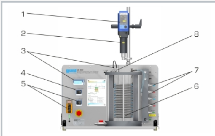
1 stirring machine, 2 torque measurement, 3 electrical conductivity measurement, 4 temperature setting, 5 flow rate setting for gas, 6 coiled tube, 7 connections for hot and cold water and gas, 8 free connections for other measuring instruments
