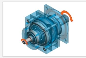
Transparent sectional view of the assembled gear
