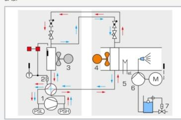
Simulated air conditioning system: 1 compressor, 2 four-way valve heating/cooling, 3 outer air fan, 4 room air fan, 5 auxiliary heating, 6 humidifier pump, 7 humidifier solenoid valve
