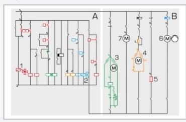
A control circuit, B load circuit; 1 four-way reversing valve heating/cooling, 2 humidifier solenoid valve, 3 compressor, 4 room air fan, 5 auxiliary heating, 6 humidifier pump, 7 outer air fan
