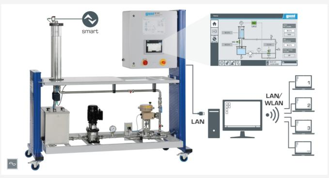
Control and operation via touch screen or a PC with GUNT software. Observation and analysis of the experiments at any number of workstations via LAN/WLAN.
