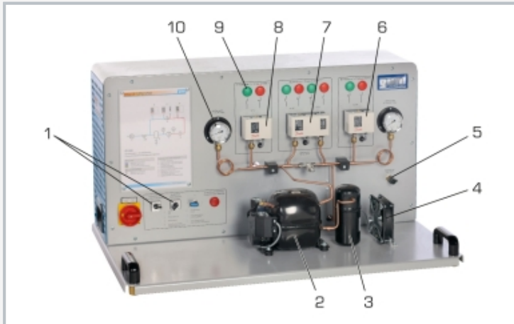
1 controls, 2 compressor, 3 receiver, 4 fan, 5 vent valve, 6 high pressure switch, 7 combined pressure switch, 8 low pressure switch, 9 signal lamps for switching state, 10 manometer
