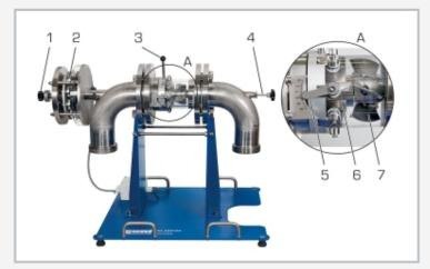
$1\,$  handwheel for adjusting the brake,  $2\,$  eddy current brake,  $3\,$  adjustment of the guide vane position,  $4\,$  handwheel for adjusting the blades;
