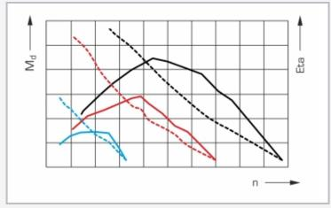
Efficiency and torque (dashed lines) depending on the speed at different angles of the blades and quide vanes:
