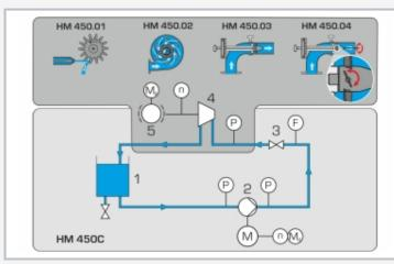
1 tank, 2 pump, 3 flow control valve, 4 turbine, 5 brake, M motor; F flow rate, P pressure, n speed, Md torque
