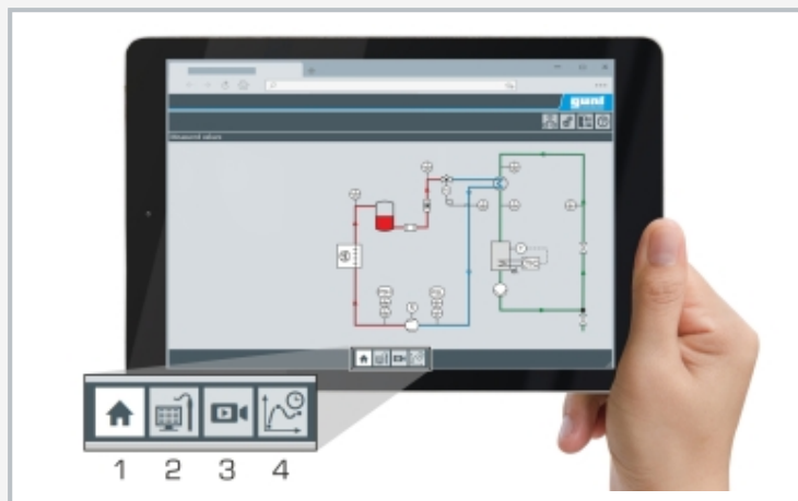
Screenshot of the web browser representation shown by example of ET 400: start screen 1 start screen with process diagram, 2 current measured values, 3 live stream, 4 graphical visualisation of experimental results
