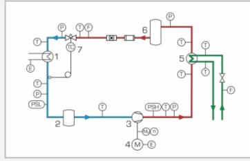
1 evaporator, 2 liquid separator, 3 compressor, 4 drive motor, 5 condenser, 6 receiver, 7 expansion valve;
