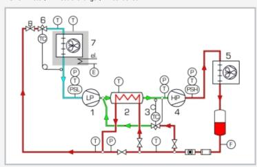
1 LP compressor, 2 intercooler, 3 reinjection valve, 4 HP compressor, 5 condenser, 6 expansion valve, 7 evaporator; T temperature, P pressure, E electrical power, F flow rate, PSL, PSH pressure switch
