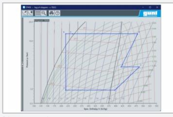
Software screenshot of a real system process 1-2 LP compression, 2-3 intercooling, 3-4 HP compression, 4-5 condensation, 5-6 supercooling, 6-7 expansion, 7-1 evaporation
