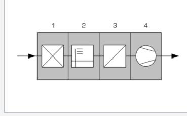
Schematic setup of the air conditioning system in accordance with DIN 1946 1 air cooler, 2 air humidifier, 3 air heater, 4 fan
