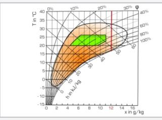
h-x diagram with comfort zone (green) and limit of comfortable humidity (red; x=12g/kg); h enthalpy, x absolute air humidity, T temperature,  $\phi$  relative air humidity
