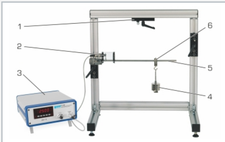
1 fixture, 2 strain gauge measuring point, 3 measuring amplifier, 4 weight, 5 bending bar, 6 adjustable rider
