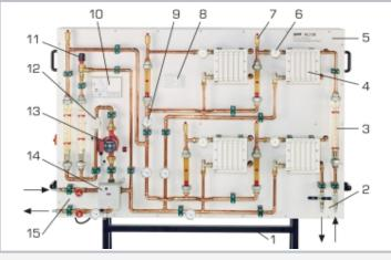
1 frame, 2 cold water connections, 3 rotameter, 4 radiator, 5 panel, 6 thermostatic valve, 7 bleed valve, 8 room temperature sensor, 9 bimetallic thermometer, 10 heating controller, 11 overflow valve, 12 feed flow temperature sensor, 13 pump, 14 mixing valve, 15 boiler water connections
