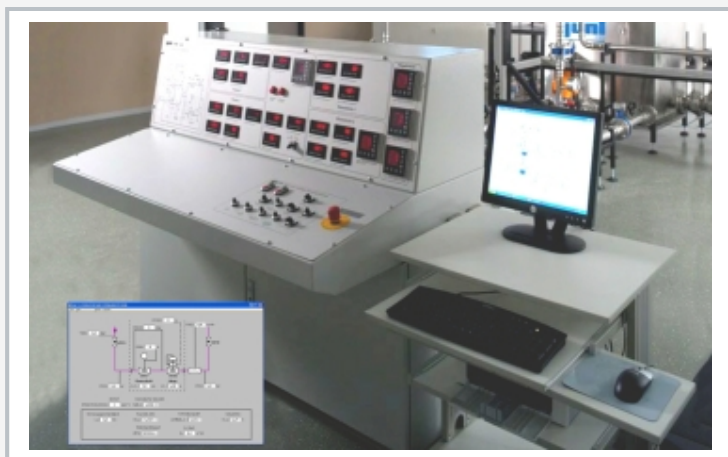
Control station consisting of control console and data acquisition for convenient recording and analysis of the experiments
