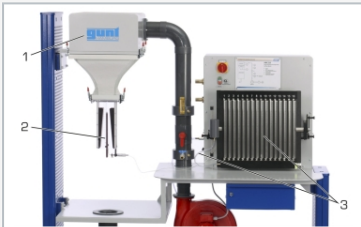
Experimental setup: 1 HM 225, 2 HM 225.02, 3 tube manometers (HM 225) with connection to HM 225.02
