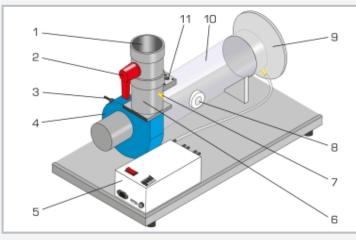
1 air outlet, 2 throttle valve for adjusting the air flow, 3 measuring point for temperature, 4 fan, 5 switch box with pressure transducer, 6 delivery pipe, 7 measuring point for pressure, 8 connector for accessory HM 240.04 / HM 240.06, 9 air inlet, 10 intake pipe, 11 connector for Pitot tube HM 240.03
