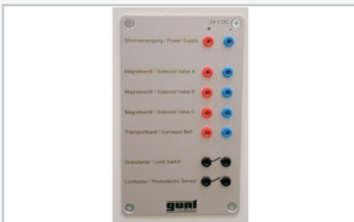
Electrical connections of the solenoid valves and sensors
