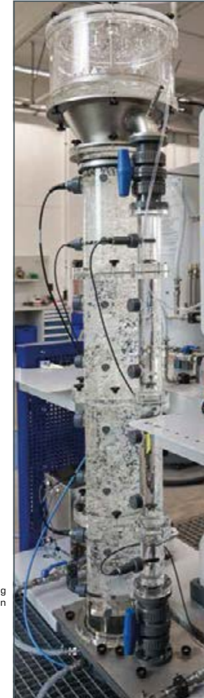
Various distributors for aerating the reactor
