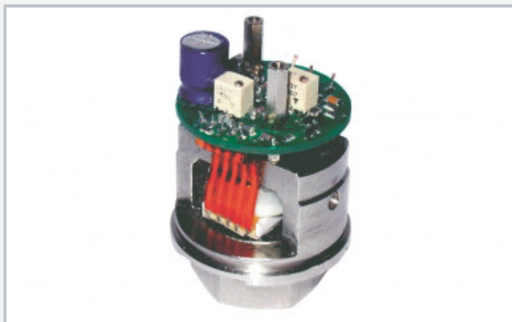
Interior layout of an electronic pressure sensor
