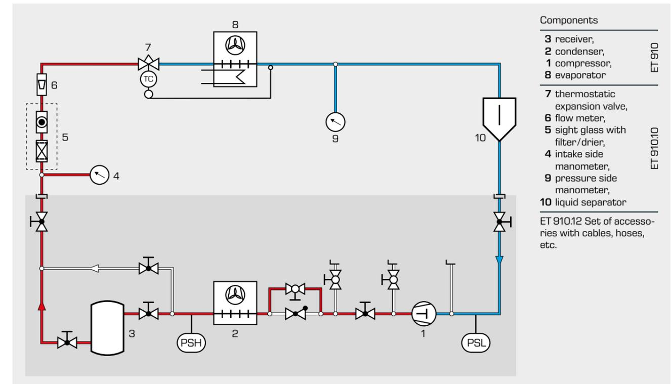
In this introductory experiment, a simple refrigeration circuit is set up, consisting of a condensing unit (compressor 1, condenser 2, receiver 3), refrigeration chamber with evaporator 8, thermostatic expansion valve 7 and sight glass with filter/drier 5.
