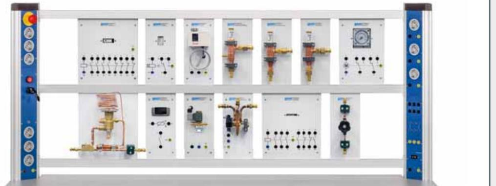
Further experiments with primary and secondary controllers in the refrigeration circuit. Electrical components can also be used to study tasks in the field of electrical engineering.
