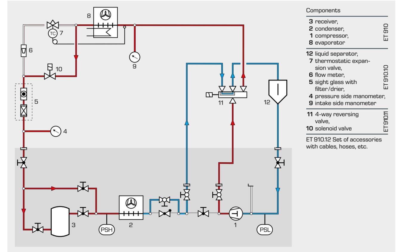
At evaporation temperatures of less than 0°C, e.g. in deep-freeze systems, the air is cooled below its dew point temperature, causing condensate to escape and freeze on the surface of the evaporator. This layer of ice hinders convective heat transfer and reduces the heat transfer surface. In addition to the option of using a time-controlled defrost heater, ET 910 also offers hot gas defrosting.
