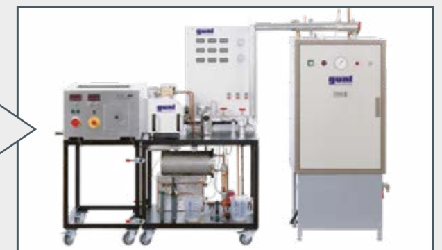
Steam power plant with 2-cylinder steam engine and electrical steam generator
