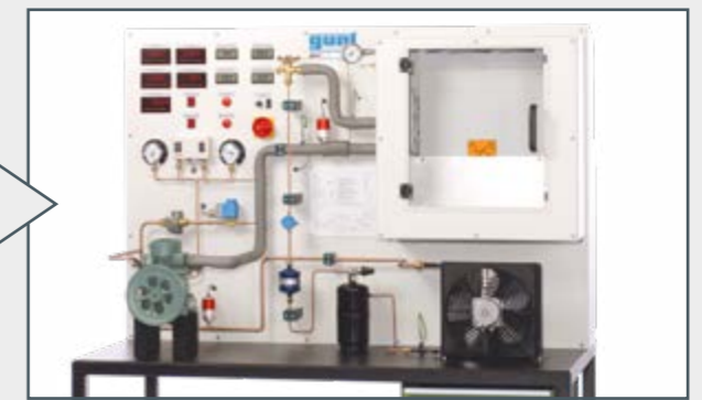
Refrigeration system with open compressor
