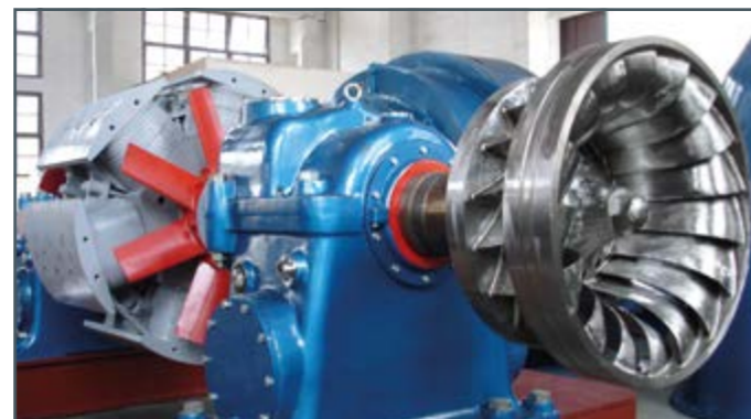
Francis turbine, deinstalled
