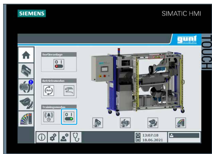
Switch on training mode on the touch screen. Operating hours counter is located in the PLC. The maintenance intervals for the various sub-systems can be simulated , i.e. adjusted.
