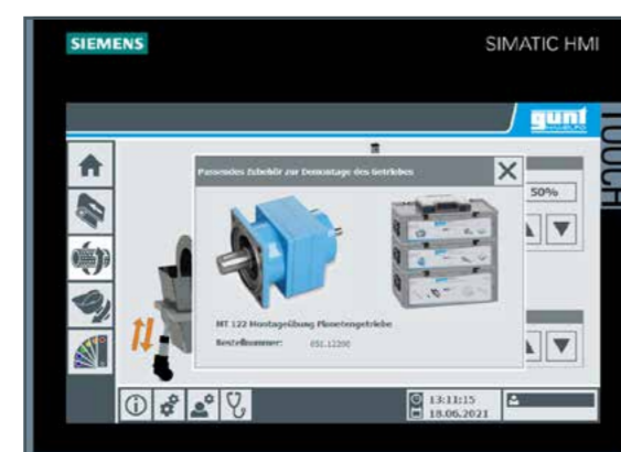
Here we suggest familiarising yourself with the planetary gear installed in the drum screen better as a separate assembly exercise.
