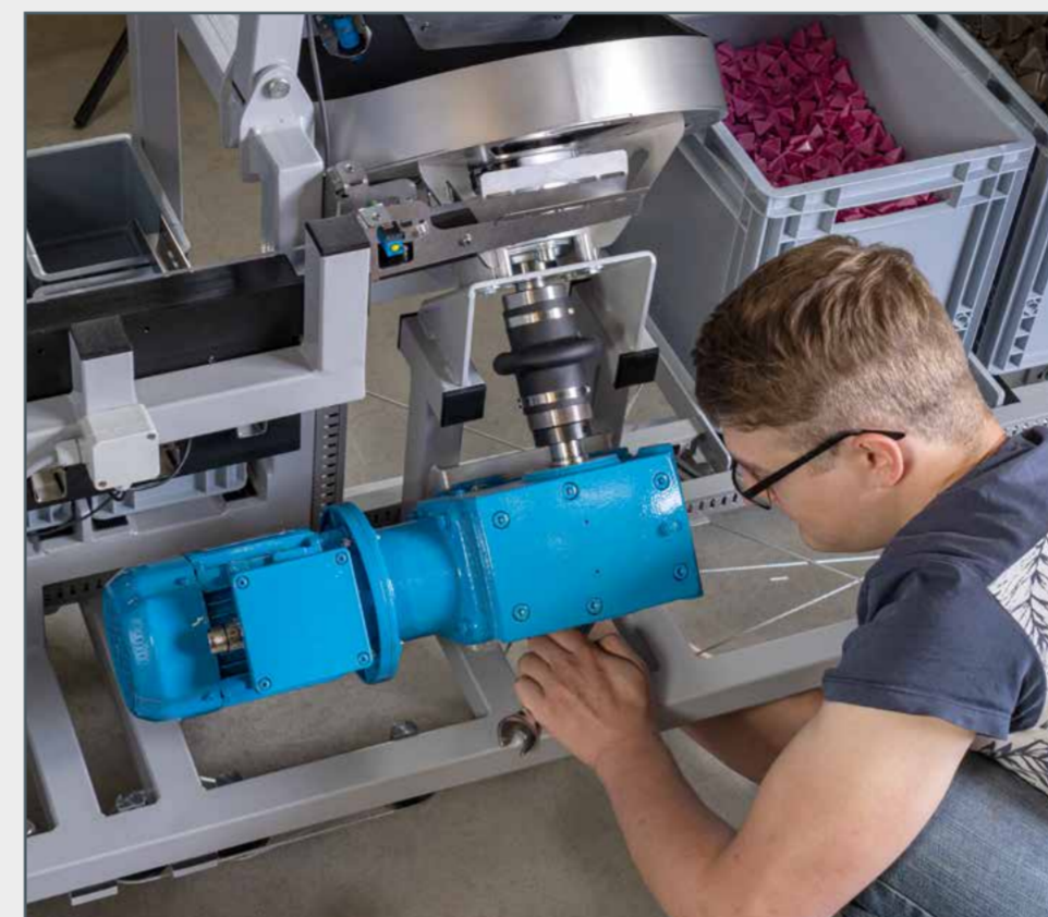
undo the threaded joint between the drive train and the frame in MT174
