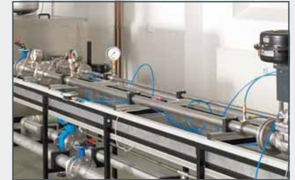
Pipe sections with different diameters and made from different materials are available for measuring pressure losses. In addition to hydraulically smooth pipe sections there is also a pipe section with a defined roughness.
