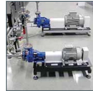
There are two different sized centrifugal pumps available for investigations on pumps.
