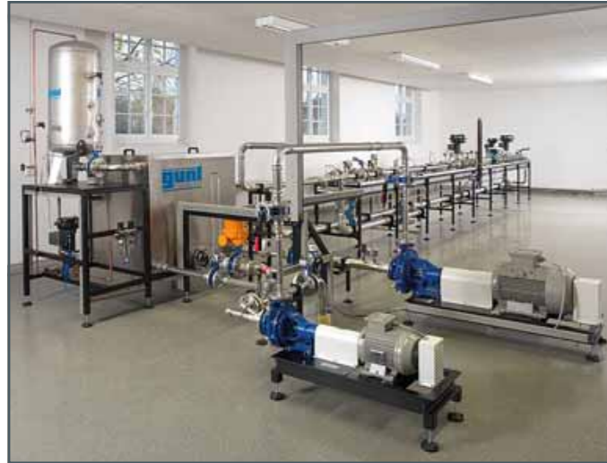
HM 124 experimental plant in laboratory with optional pressure controlled system via a pressure vessel
