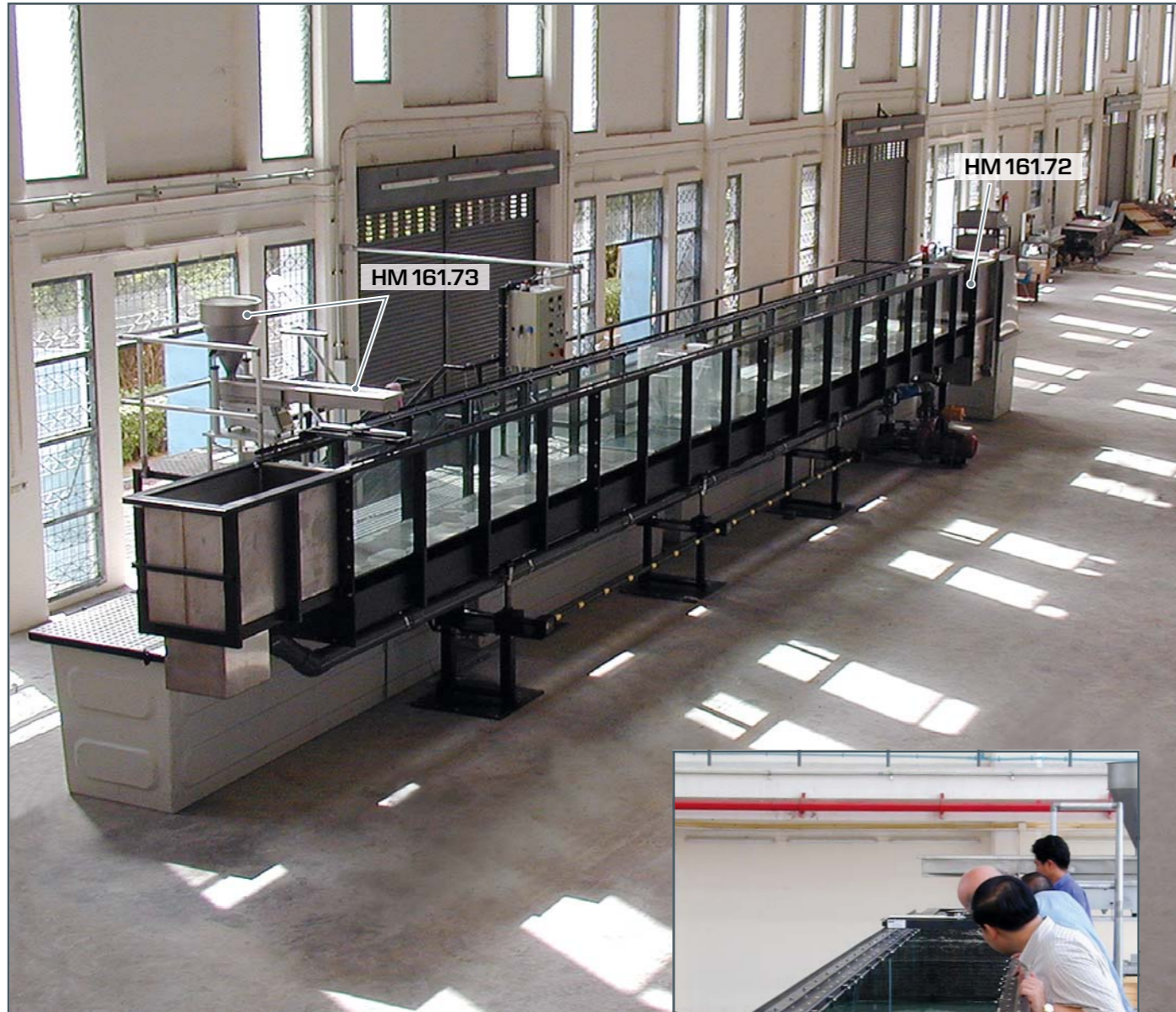
Experimental flume HM 161 with sediment transport. The sediment feeder HM 161.73 sits on the inlet element. At the end of the experimental section, the sediment trap HM 161.72 separates the sediment.
