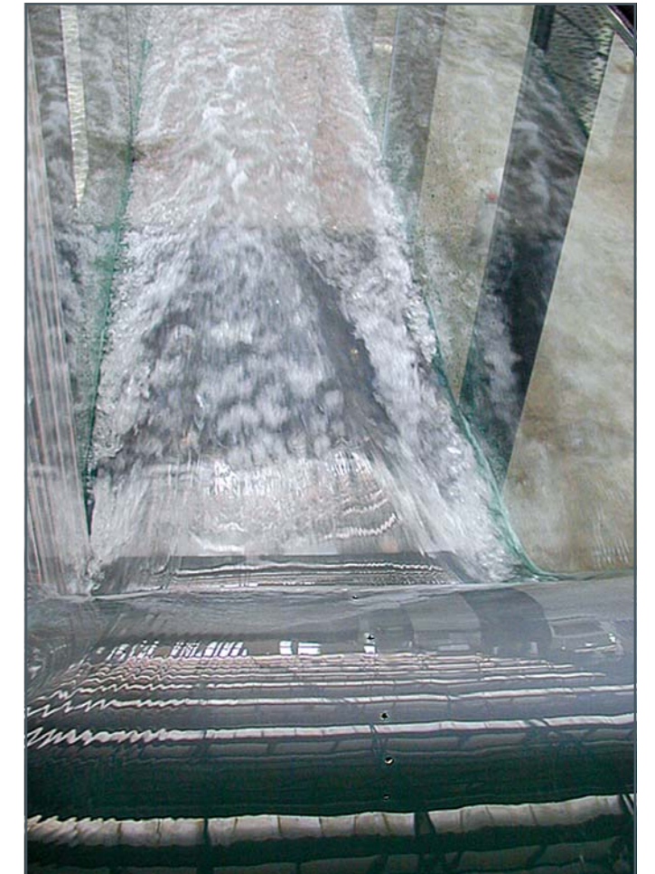
Plan view during discharge over the ogee-crested weir HM 161.34
