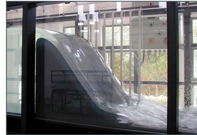
Side view during discharge over the ogee-crested weir HM 161.34
