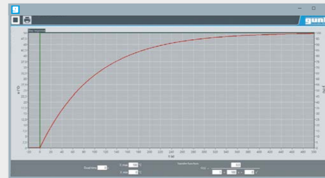
Controlled system with PT 1 behaviour
