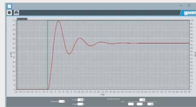
Controlled system with PT 2 behaviour
