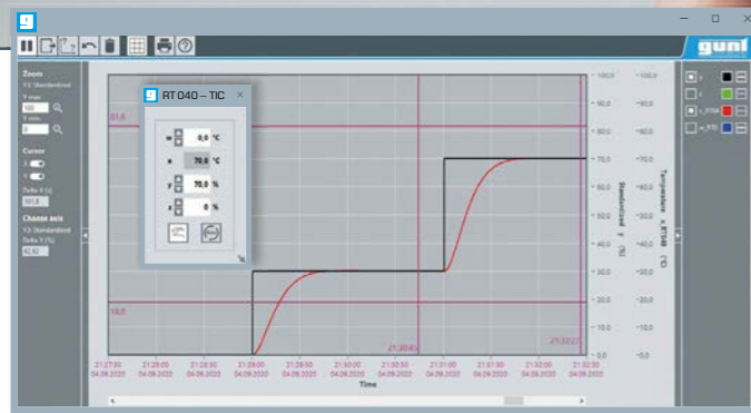
The simulation function in the GUNT software can also be used to investigate control engineering issues for which no real system is available.
