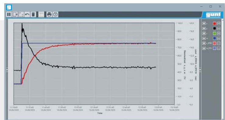
Level control with PID controller, reference variable step
