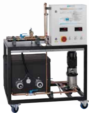
WL 312.10 Hot water generator
