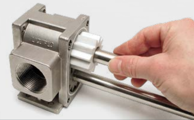
MT 186 Assembly & maintenance exercise: gear pump
