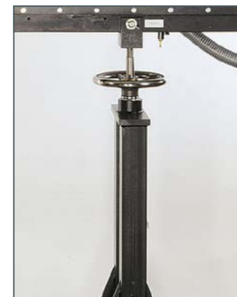
Electrical inclination adjustment in HM161
