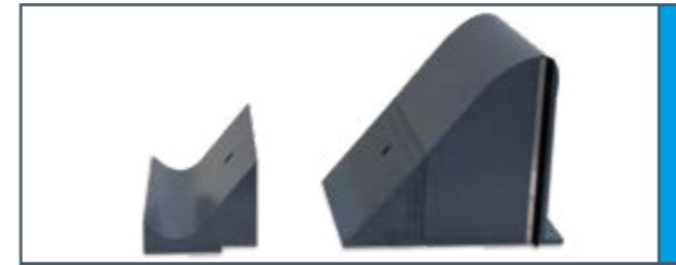
HM 162.32 Ogee-crested weir with two weir outlets
