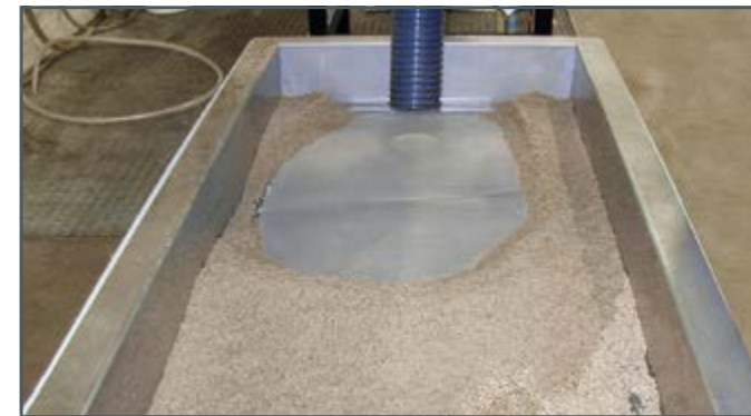
Sediment trap HM 160.72 in the water tank of HM 160 for collecting the sediment
