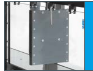
HM 162.29 Sluice gate
