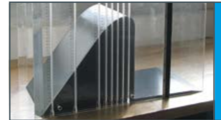
HM 162.34 Ogee-crested weir with pressure measurement
