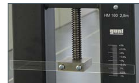
Inclination adjustment in HM162 and HM163: left manual, right electrical inclination adjustment HM162.57
