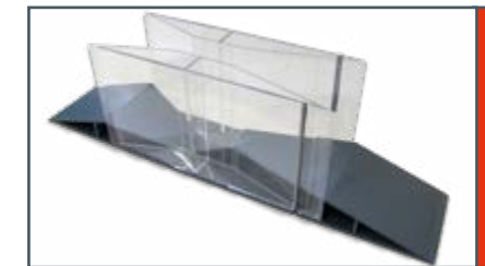
HM 162.55 Canal Parshall
