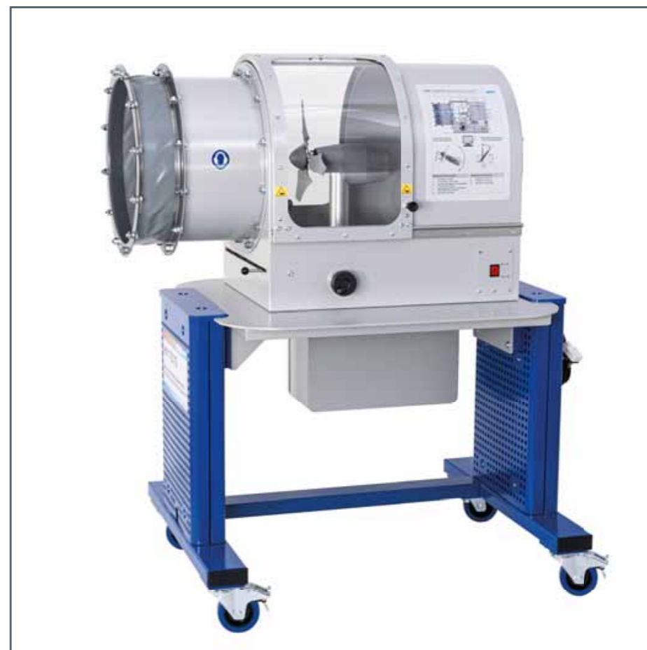
HM 170.28 Measurement of the wake of a cylinder immersed in a flow and demonstration of a wake depression, wake rake consisting of 15 Pitot tubes
