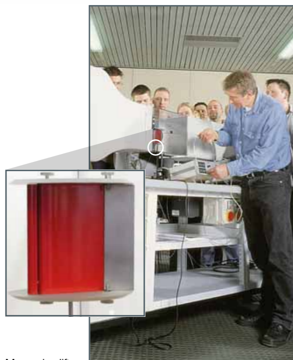
Measuring lift and drag forces as a function of the angle of attack of an aerofoil with flap and slot
