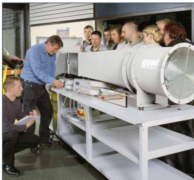
Training at the HM 170 Open wind tunnel at the Technical College for Aeronautical Engineering in Hamburg (Germany)
